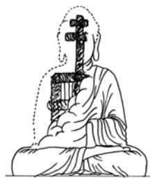
Fig 155 Wooden core and clay model construction
